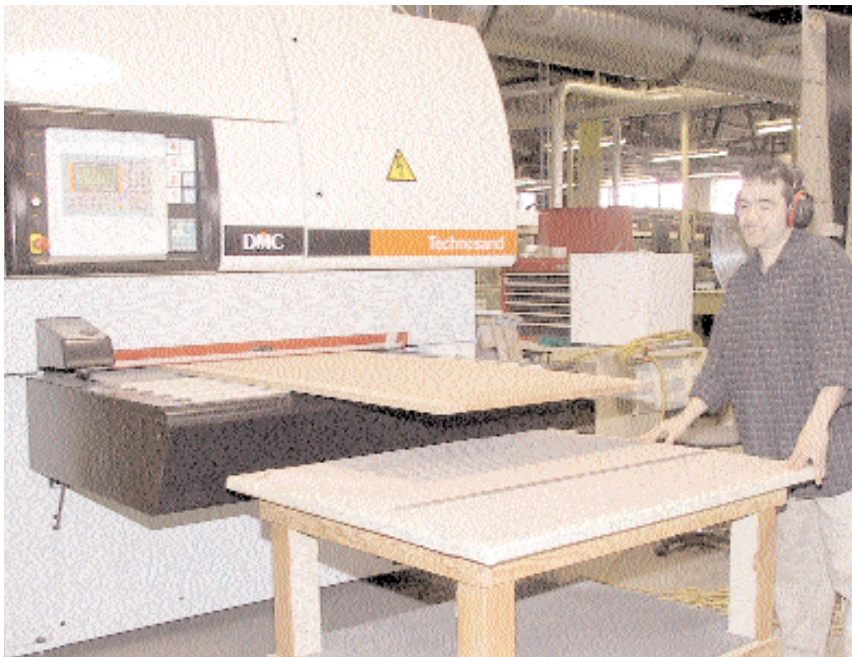
The DMC sander by SCM Group is an example of modern equipment at Barsanti that benefits from a stable air pressure supply.
